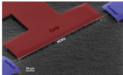
SiN nanostring 300 μm long, 300 nm wide, 190 nm thick (gate not used)
