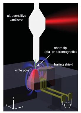
Artistic rendering of the experiment performed. An ultrasharp diamond needle is attached to the end of a cantilever that serves as a highly sensitive mechanical detector. We scan the needle over the surface of a commercial write head device and record the forces between the diamagnetic polarization in the diamond and the pulsed magnetic field gradient generated by the write pole.
