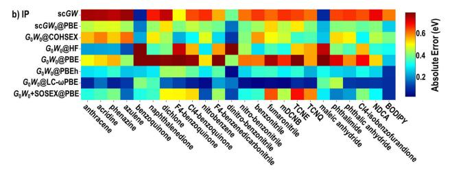
Heat map representation of the absolute errors in eV with respect to CCSD(T) of different *GW* approximations for the ionization potentials of the benchmark molecules<sup>2</sup>.
