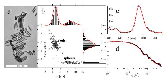
The three techniques at a glance for one sample. (a) Selection from a TEM image. (b) TEM analysis : aspect ratio vs. radius for all analyzed particles, with histograms of both parameters. The solid lines are Schulz distributions. (c) Absorbance spectroscopy data and (d) SAXS data for the same sample.
