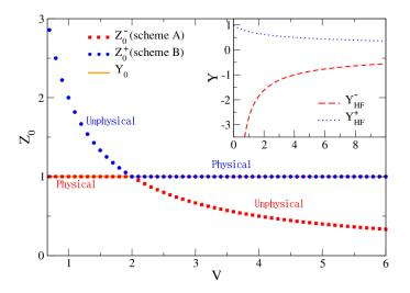
The noninteracting Green's function  $Z_0$  as a function of the interaction V obtained in a simple one-point model using two different iteration schemes (**A** and **B**). Squares (red):  $Z_0^-$ , the solution of scheme **A**; circles (blue):  $Z_0^+$ , the solution of scheme **B**; continuous line (orange):  $Y_0$ , the physical noninteracting Green's function
