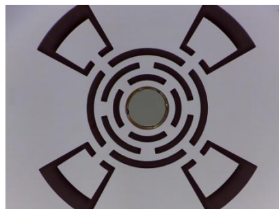
SEM image of the micro-mechanical device with the central, 0.4 mm diameter, mirror.
