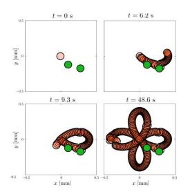
Simulation of the trajectory of one bubble (with a diameter of 50  $\mu$ m, in pink) driven by an actuator consisting of two fixed pulsating bubbles (with diameters of 53  $\mu$ m and 55  $\mu$ m respectively, in green).
